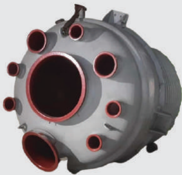
PFA Coated Vessel With Welded Baffles
